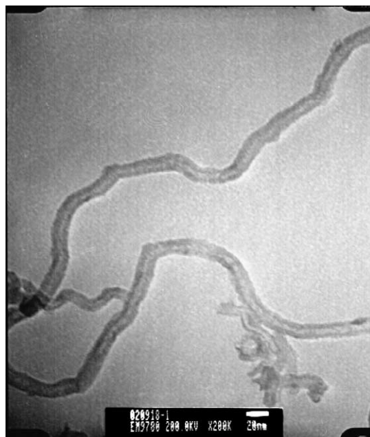
Fig. 2. TEM micrographs of purified multi-walled carbon nanotubes.
